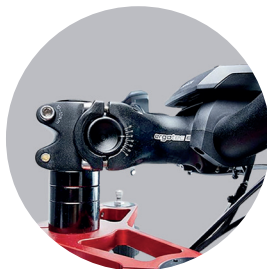
Steering damper additionally stabilises the handling
